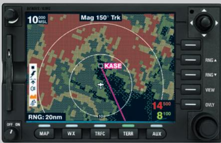
The Bendix/King KGP 560 and KGP 860 Enhanced Ground Proximity Warning Systems for General Aviation (GA-EGPWS) enhance situational awareness by incorporating the latest technology, including GPS position and a terrain and obstacle database, to give you a clear picture of the terrain ahead.
