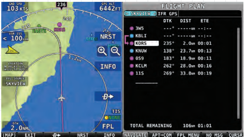
SkyView's navigation engine flies like you would. It anticipates waypoints and turns just before them to avoid needless overshoots. You can even display the graphics and waypoints from external IFR GPS flight plans.
