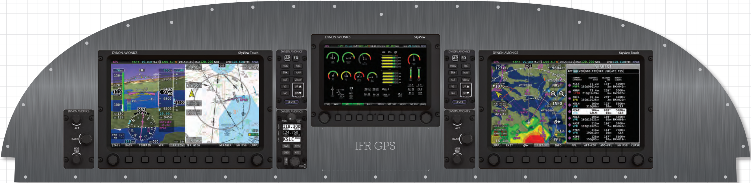
With three displays, you're actually equipped better than many airliners. We like to fly with the PFD and Map on the pilot's D1000, with the engine instruments on the 7" D700.
