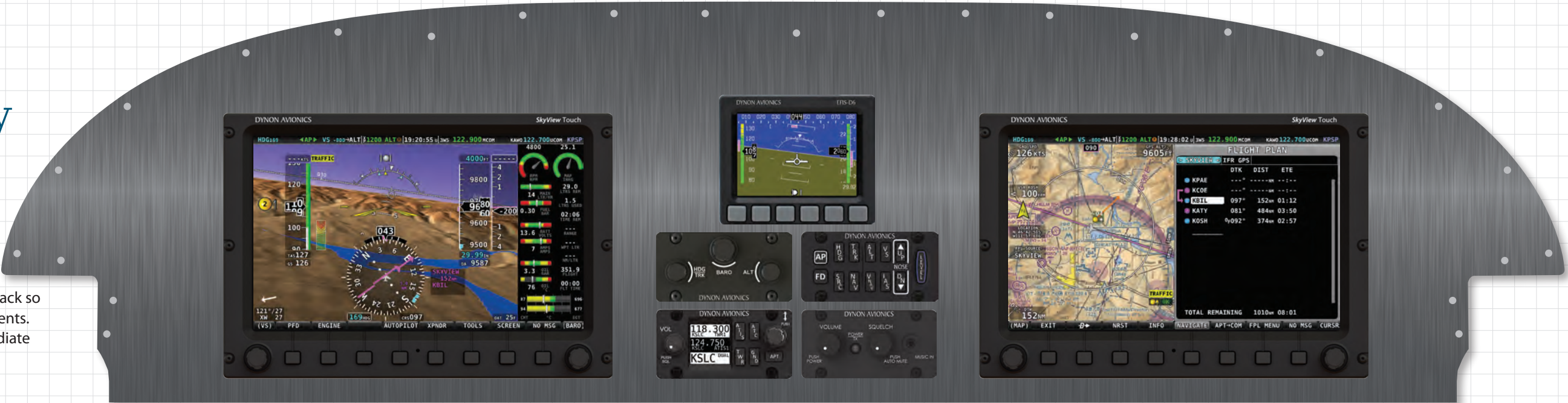
A Dynon EFIS-D6 offers an inexpensive independent backup set of flight instruments.
